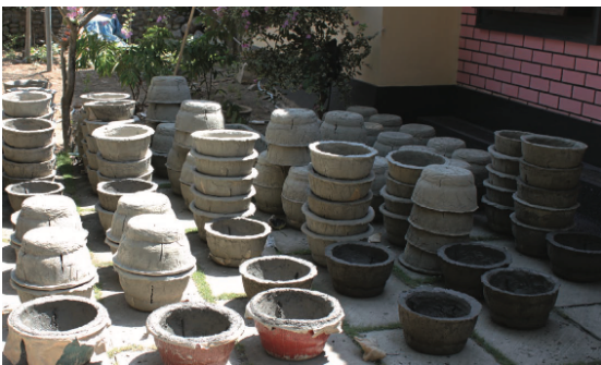
Figure 4: Artificial reef structures ready for installation Photo: James Frey
